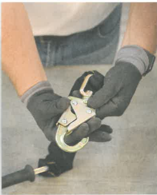
FIGURE 44 Inspecting the snap hook
