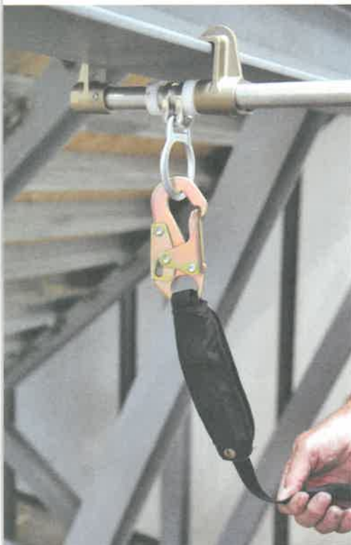
FIGURE 5 Lanyard attached to a movable beam slide
