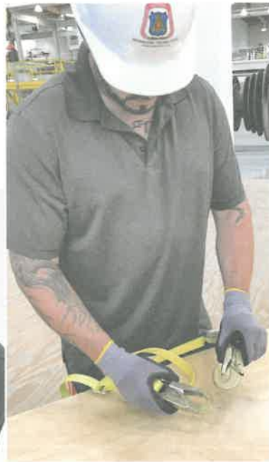
FIGURE 33 Inspecting the snap hooks
