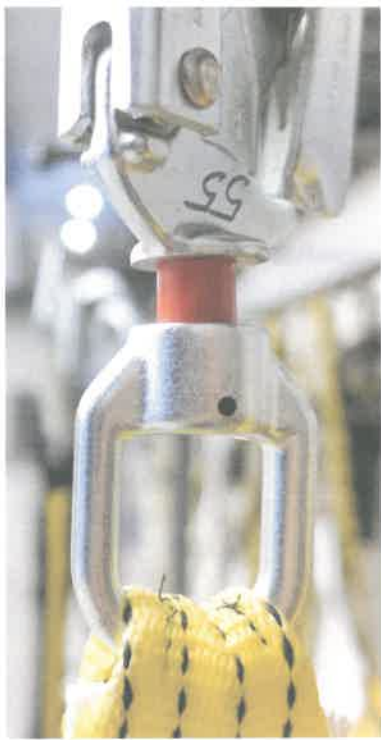
FIGURE 33 Inspecting the snap hooks
