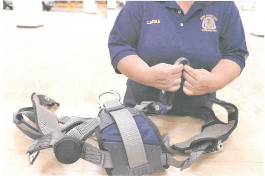
FIGURE 10 Inspecting a PFAS
