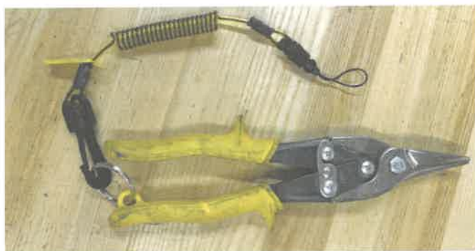
FIGURE 35 Tool retrofit with tether tape
