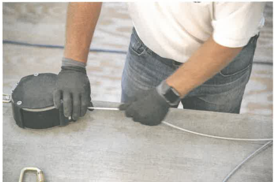
FIGURE 46 Inspecting a length of the lifeline
