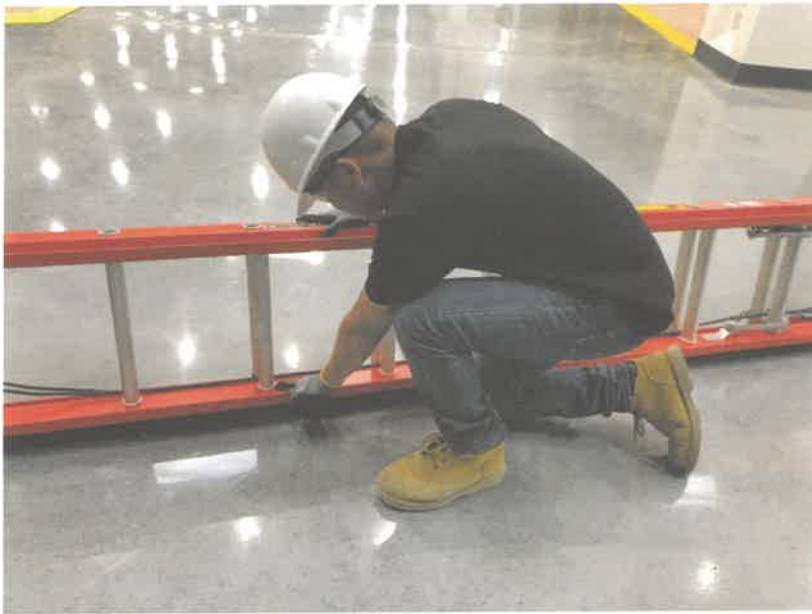
FIGURE 17 Inspecting a rung-to-rail connection
