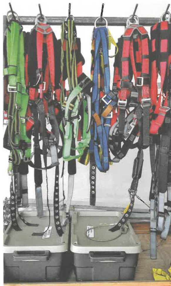
FIGURE 59 Properly hung harnesses
