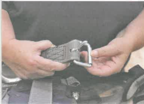
FIGURE 15 Inspecting the buckle attachment
