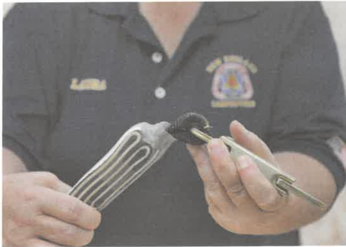
FIGURE 28 Inspecting the shock absorber pack
