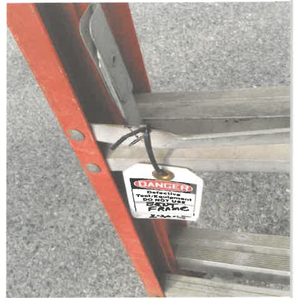
FIGURE 18 Damaged ladder with warning
