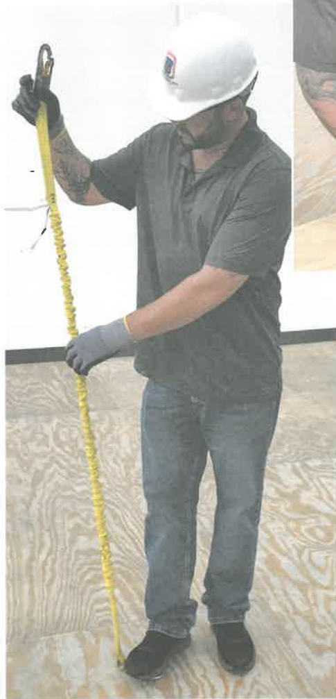
FIGURE 35 Inspecting a shock-absorbing stretch lanyard
