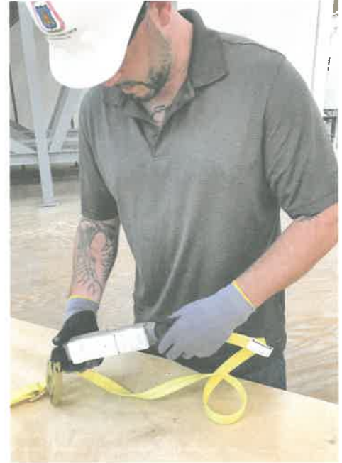
FIGURE 34 Inspecting the shock absorber pack
