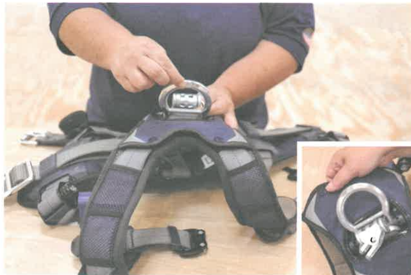
FIGURE 14 Inspecting a D-ring
