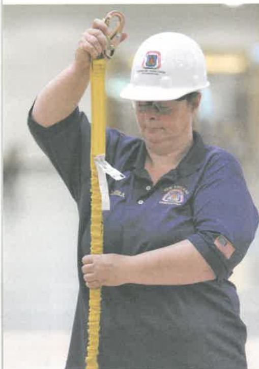
FIGURE 27 Inspecting a shock-absorbing stretch lanyard
