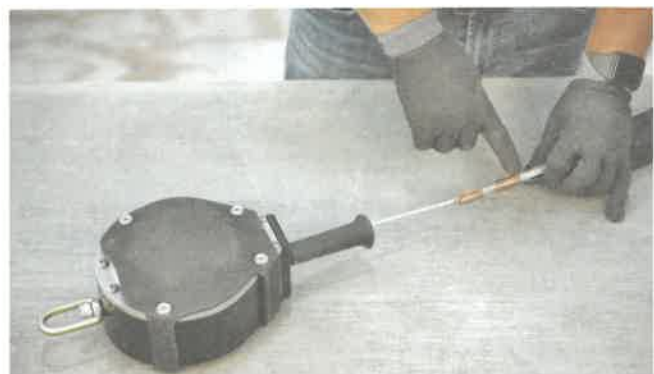
FIGURE 38 Inspecting a swage fitting on a lifeline
