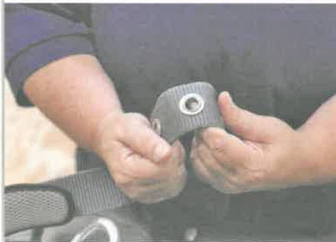
FIGURE 16 Inspecting the grommets
