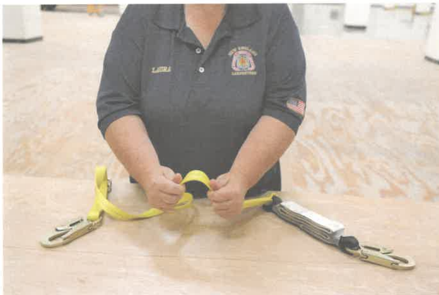
FIGURE 25 Inspecting a web lanyard
