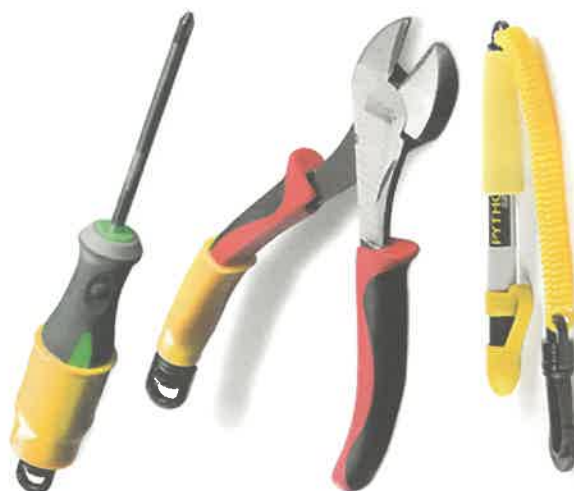
FIGURE 36 Tools retrofit with sleeve
