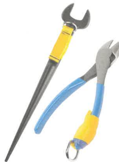
FIGURE 32 Tools retrofit with shrink-wrap
