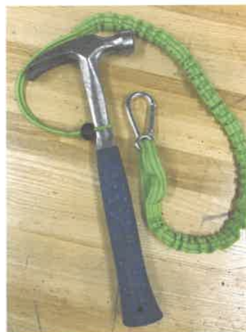
FIGURE 34 Tool retrofit with cinch
