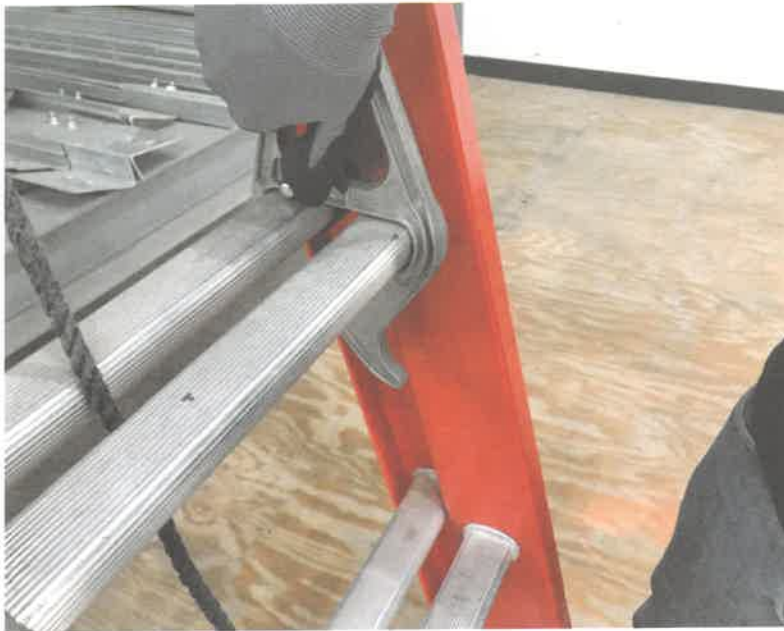
FIGURE 39 Securing the extension lock
