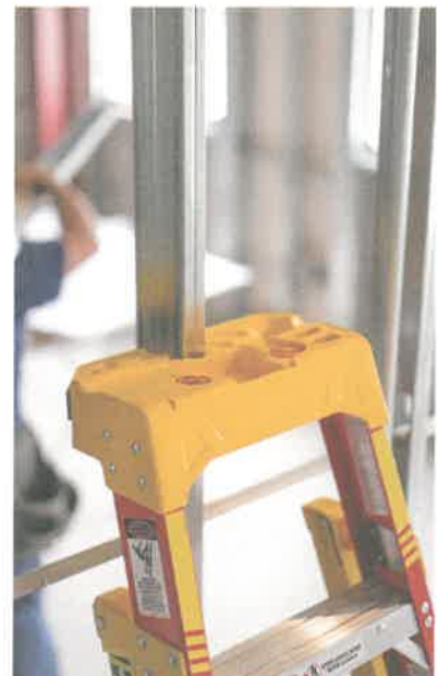
FIGURE 25 Stepladder with notch
