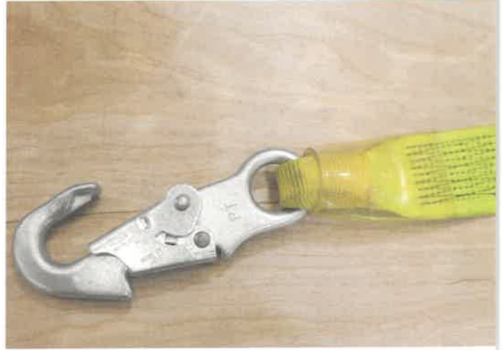
FIGURE 29 Damaged self-locking snap hook
