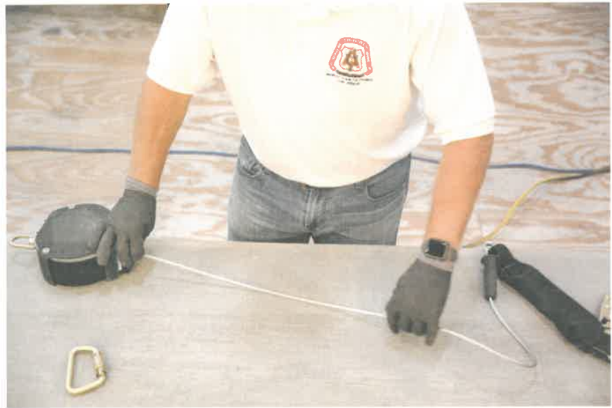
FIGURE 39 Checking an SRD for spring tension
