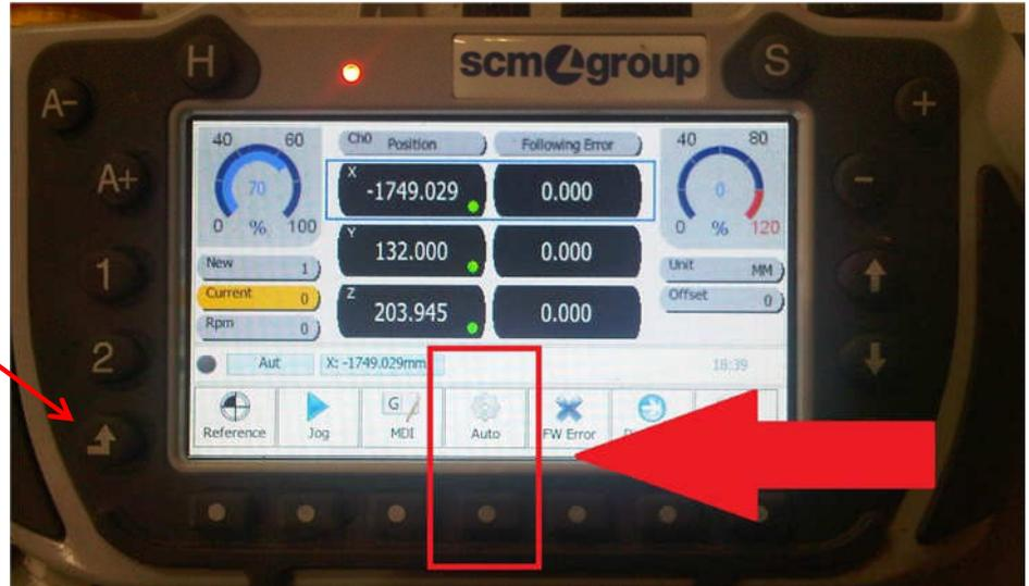
7. Press the START CYCLE button on the Sintesi Device to start the machine operation:
