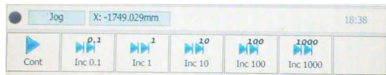
Note: The Rapid Potentiometer controls the jog speed. Select Continuous or incremental Jog with the bottom buttons.
