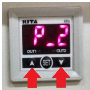
906. Press “SET” to save the new setting and display “P3”. P3 and P4 are not used by the Pratix S.
