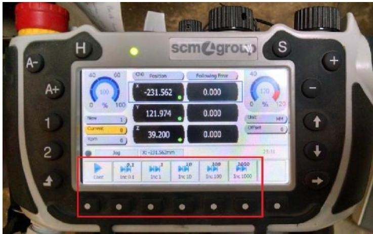
1004. Turn the Axis Speed Adjustment Potentiometer (Rapid Speed Turret) to adjust movement speed. The meter on the top left of screen will reflect the changes (100% equals 25 m/min (82 ft/min)).
