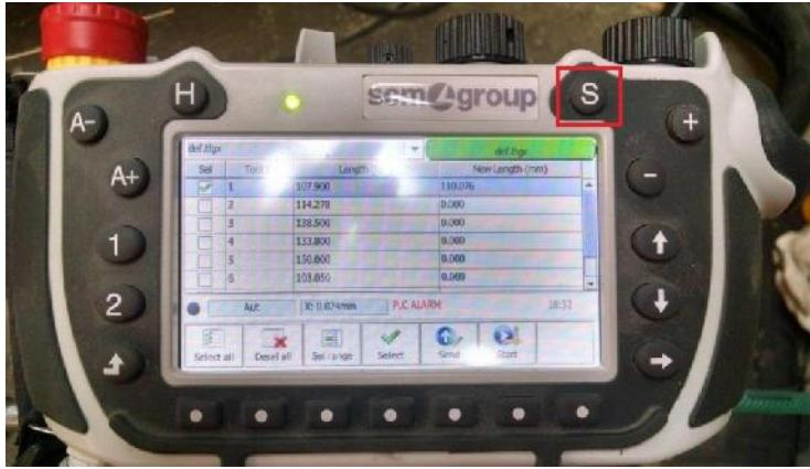
710. The Sintesi will display a value in the “New Length (mm)” column. This is the length of the tool.
