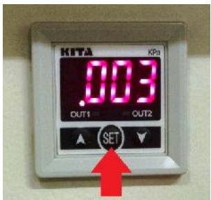
905. Press the “UP” or “DOWN” Button to adjust “P2”.
