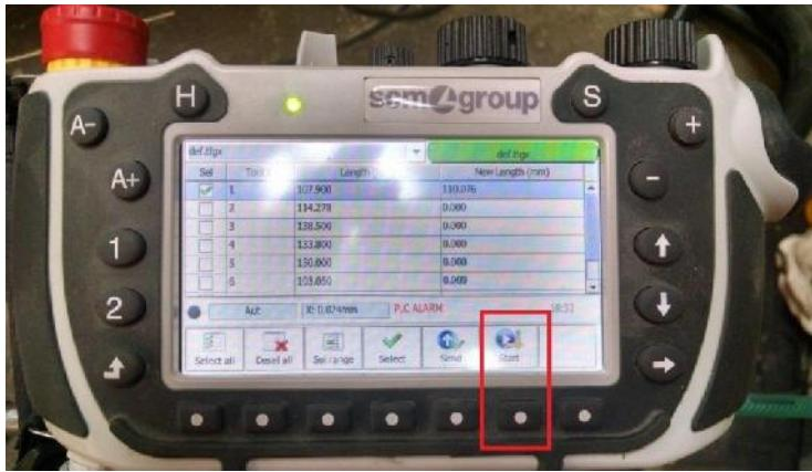
709. Then Press the “START CYCLE (S)” Button to measure the tool.
