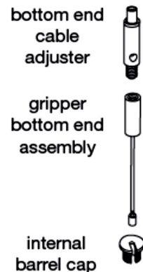
Figure 53 - Bottom End Cable Assembly
