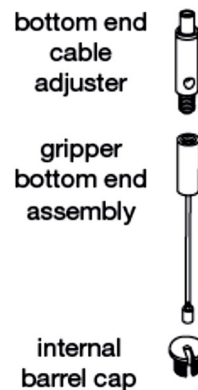
Figure 53 - Bottom End Cable Assembly
