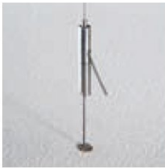
Figure 51 - Completed Cable End Assembly
