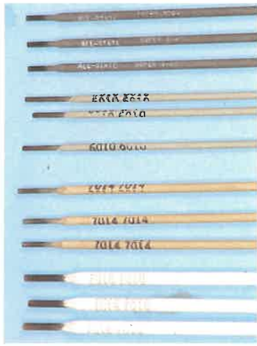
FIGURE 6 Location of the electrode classification number
