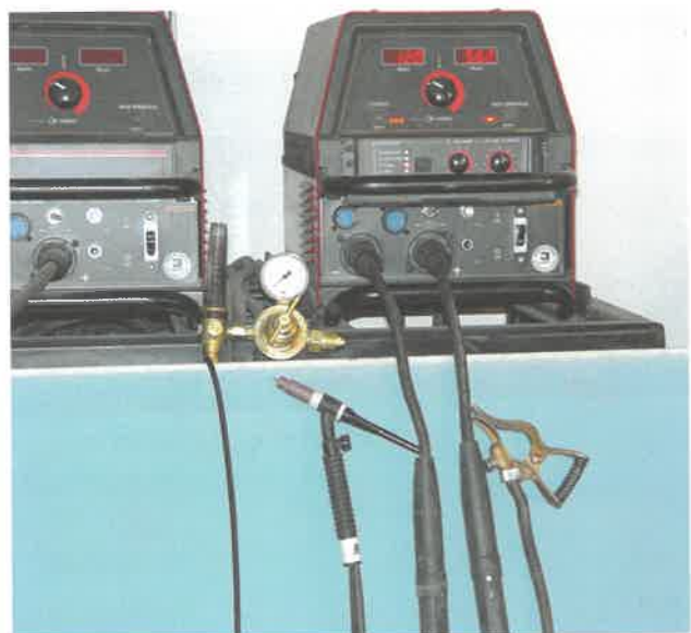
FIGURE 5 Machine in DCEN
