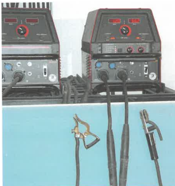
FIGURE 4 Machine in DCEP
